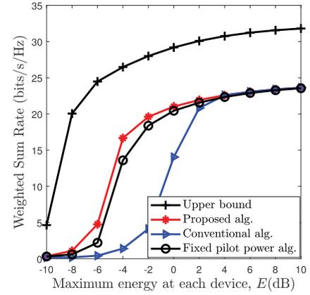
Fig. 9. Average weighted sum rate vs. maximum energy limit  $10\log_{10}E$  for various schemes for the case of MRC.
