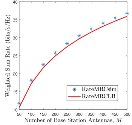
Fig. 5. Tightness of the derived data rate LB for the MRC case.
