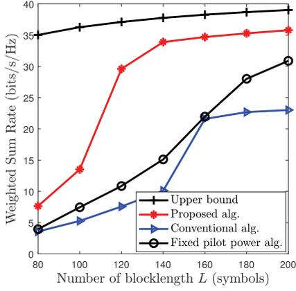
Fig. 14. Average weighted sum rate vs. blocklength for various schemes for the case of ZF.
