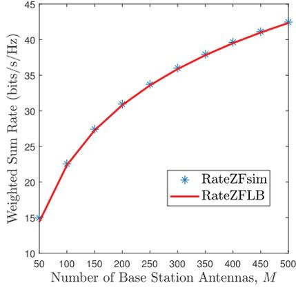
Fig. 6. Tightness of the derived data rate LB for the ZF case.
