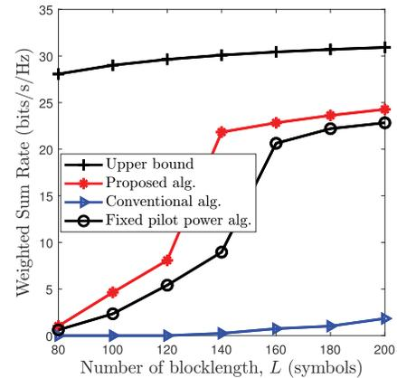
Fig. 13. Average weighted sum rate vs. blocklength for various schemes for the case of MRC.
